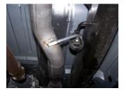
**2.** Install head pipe #A onto your existing stock front pipe and attach with clamp #F. Use a jack stand to support the converter. Insert welded hanger into rubber grommet.
