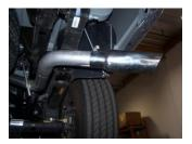
**6.** Install exit pipe #D onto overaxle tail pipe. Use clamp #F to secure. DO NOT TIGHTEN.
