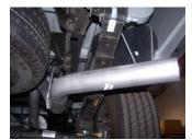
**5.** Install the overaxle tailpipe #C into the muffler 1½"-2". Use clamp #F to secure tailpipe to muffler. DO NOT TIGHTEN. Insert welded hanger into rubber grommet.
